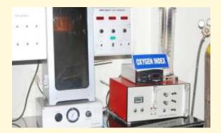
Visibility during burning (3m<sup>3</sup> Test) as per IEC 61034 Part-I & BS 7622
