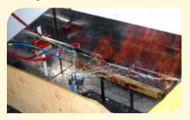
Category Z · Exposure to Fire with Mechanical Shock at 950° C as per BS 6387
